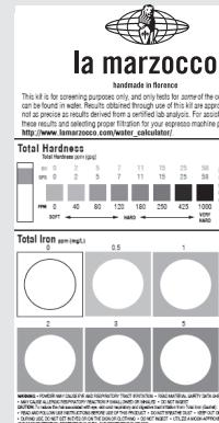
In order to enable you to check if your water supply is within the suggested ranges, La Marzocco machines will be equipped with a quick water test kit (see image below) including 6 test-strips and instruction cards. The parameters that you can measure are Total Hardness, Total Iron, Free Chlorine, Total Chlorine, pH & Total Alkalinity, Chlorides.
