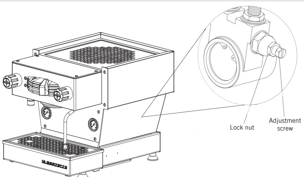
**Figure 3 - Water Pump Pressure Adjustment**
